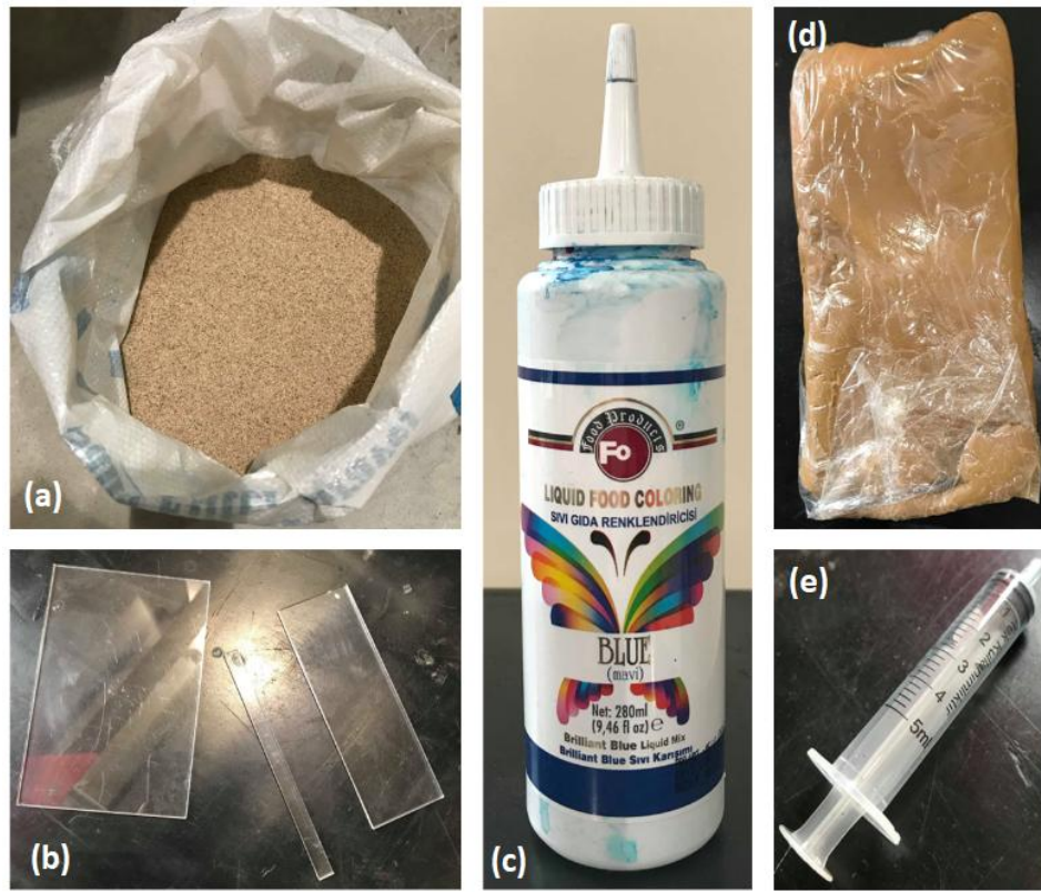
Figure 2: Material used in the experiment including (a) sand sample, (b) additional plexi-glasses, (c) food color, (d) clay, and (e) syringe.
